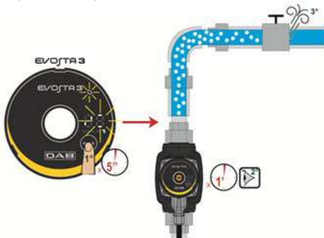
Figure 9: Automatic venting of the pump
